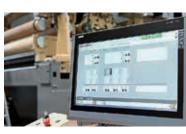
Central touchpanel (22") has a clear overview and permits complete operation of the machine from the control room.
