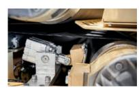
The rollers are gently stopped after a sanding belt rupture. This means that the safety doors can be opened faster.
