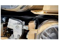
The rollers are gently stopped after a sanding belt rupture. This means that the safety doors can be opened faster.
