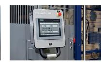
Local control panel (7") for the on-site control unit and a quick overview of all relevant process data.
